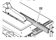
For use as rip fence the long fence extrusion (22) must be installed. It is mounted on the guide extrusion at the front of the saw table.
